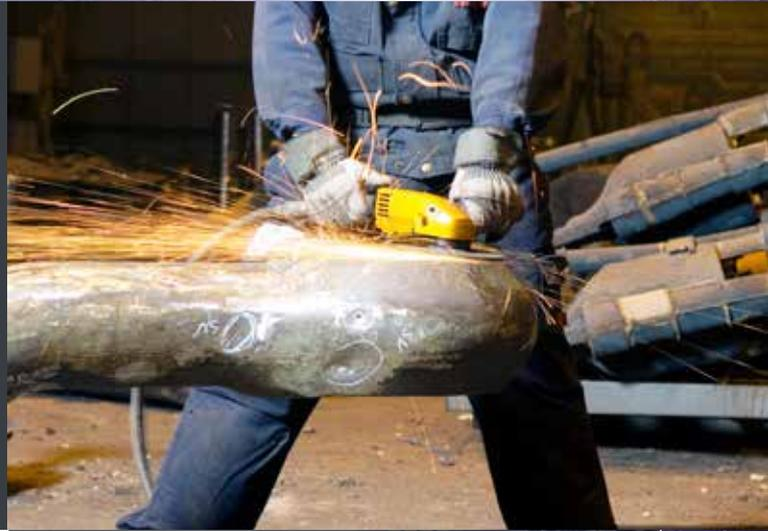
**EFFECTIVE GRINDING** with the right tool makes additional processes unnecessary. Cast remains are easily removed with rough grinding – cutting close to the work piece leaving close to nothing behind.
