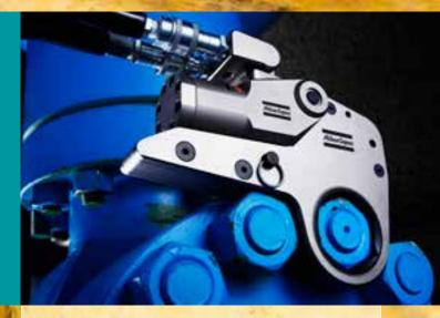
ACCESS TO NUTS AND BOLTS is a big issue on BOP's. Our solution, the RTX low clearance wrenches with corresponding link for nut size. A uni-swivel moves the hoses away from the operation. Fit it with an onside reaction arm to remove the stress off the adjacent nut.
