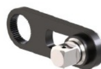
Reaction bar Sliding 1" square drive, spline type 5. CC distance 80-125 mm. Mounting: Mounted on the front gear splines. Designed to take reaction on adjacent bolt or material. 4210 4481 85
