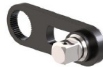
Reaction bar, sliding drive Sliding 1" square drive, spline type 5. CC distance 80-125 mm. Mounting: Mounted on the front gear splines. Designed to take reaction on adjacent bolt or material 4210 4481 85
