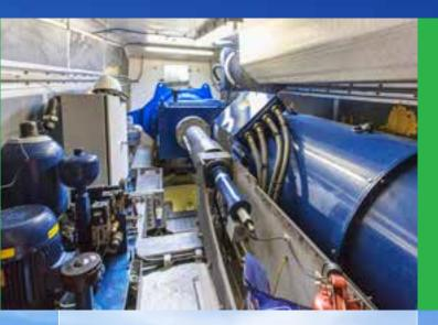
MOUNTING OFTHE GEAR BOX in the nacelle. Tensor Revo tighten 32 thread rods, M33, to 1500 Nm in controlled manner. This electric tool solution reduce noise and vibrations, and it gives a fast and accurate assembly of the gear box.
