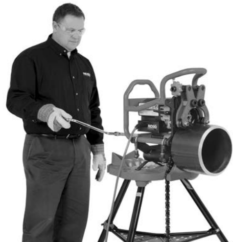
Figure 20C – Bevelling Operation (Fixed Beveller/Rotating Pipe)
