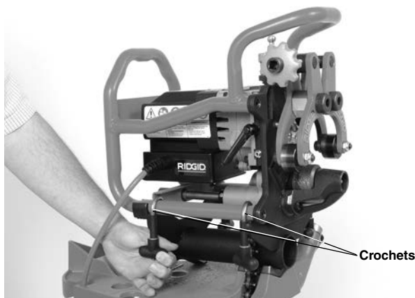
Figure 9 – Securing Beveler to Adapter
