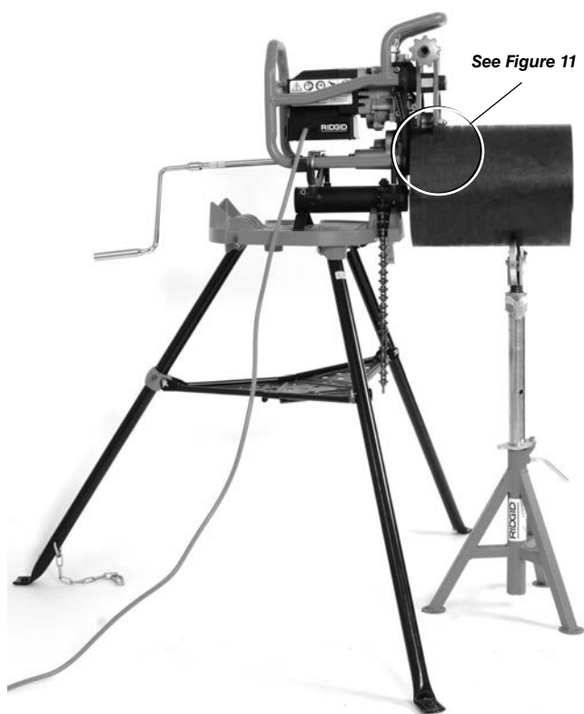
Figure 12 – Fixed Beveller, Short Pipe, One Pipe Stand
