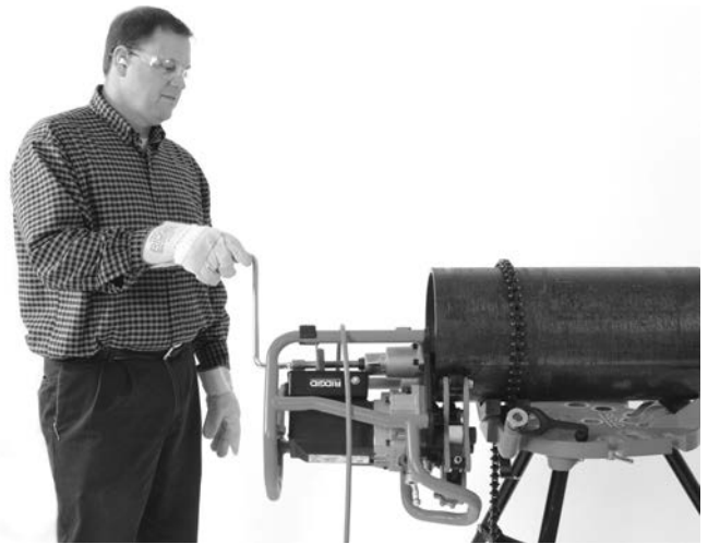
Figure 20B – Bevelling Operation (Fixed Workpiece/Moving Beveller)
