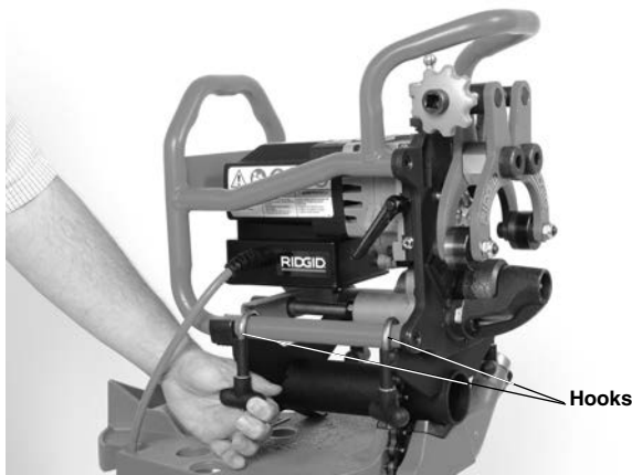
Figure 9 – Securing Beveller to Adapter
